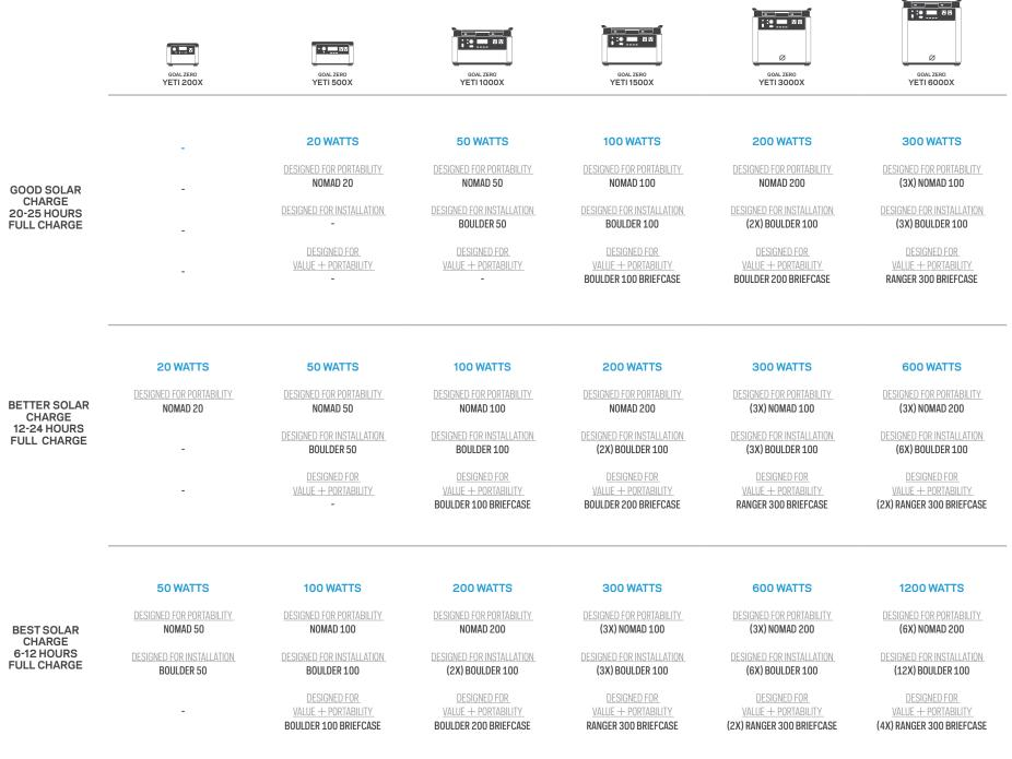
\*Charge times depicted in the "Yeti + Solar Charge Times" table assumes standard conditions of 75 degrees and 1000 watts/meter squared solar radiance. The lower end of the range requires frequent repositioning towards the sun, which results in the fastest charge times. The high end of the range presumes the panel is in a fixed position, which results in longer charge times.
